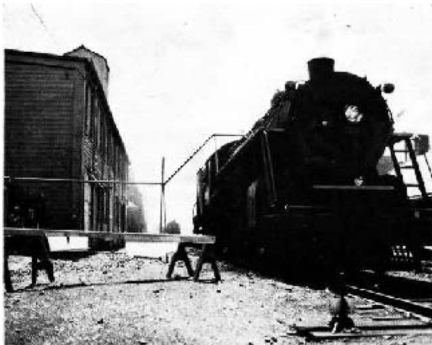
This is one of two Erie locomotives standing on a siding near the E. I. du Pont de Nemours plant in Forest avenue, Kearny, N. J., recently, with a full head of steam to keep high pressure lines at the plant in operation. Parts of the du Pont company's steam lines were temporarily shut down to permit repairs and the two engines helped maintain continuous supply of steam essential for certain chemical operations.--Newark (N. J.) News photo
