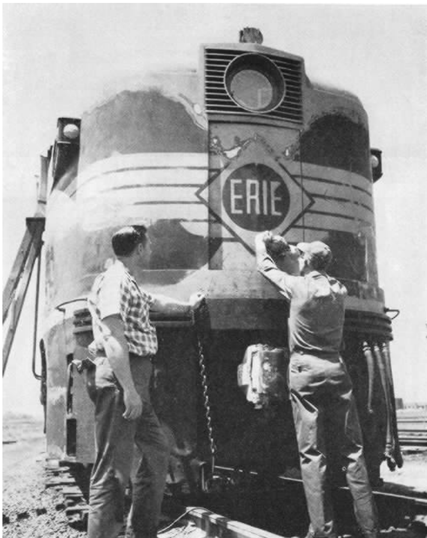
FIRST STEP: The locomotive is thoroughly cleaned and old paint sanded down. Here Holton G. Collins, foreman at Marion, and Harold E. Hoptry, painter, are at work.
