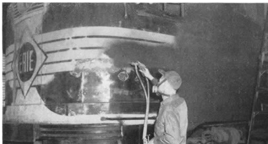
THE PRIMER COAT IS applied with a spray gun like other finishes.
