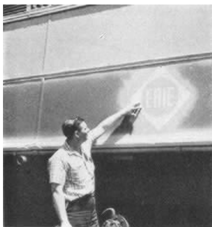
YELLOW COAT, first to be applied is inspected.
