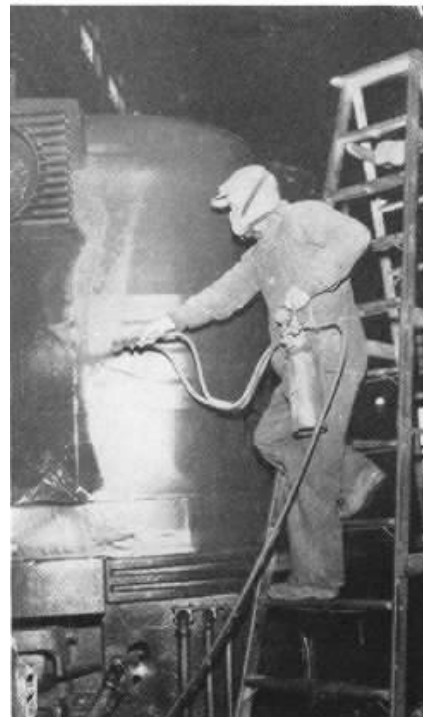
THE PRIMER COAT IS applied with a spray gun like other finishes.
