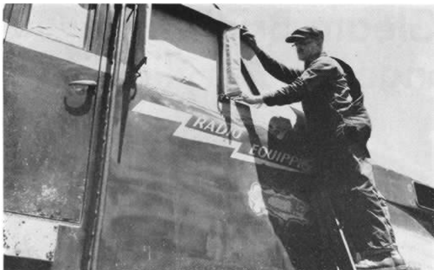
FIRST MASKING IS APPLIED to keep finish off glass surfaces.
