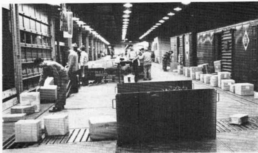
MOVING SIDEWALKS CARRY packages from Erie cars to the sorting area. The floor-level conveyors are also used in loading cars.
