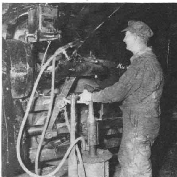
John Dick, pipefitter at Hornell backshop, recommended using an oil pump with small drum and proper fittings to fill locomotive auxiliary lubricator pipe lines with oil. Several engines can be serviced before refilling drum
