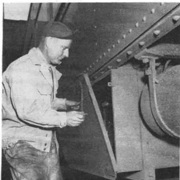
John J. Corbliss, electrician at Jersey City car shop, prevents damage to passenger car storage batteries by riveting a small piece of angle iron on ends of battery case door. Eliminates dust, cinders, snow and moisture
