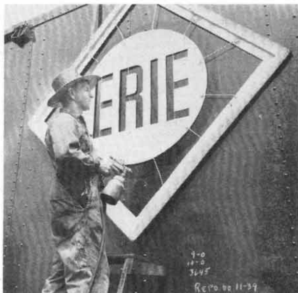
F. W. Rombausek, carman at Port Jervis, suggested substituting round in place of flat rods to tie the circle in the Erie diamond to the metal outside frame. These raised round rods allow the paint to be sprayed under them, eliminating any hand painting
