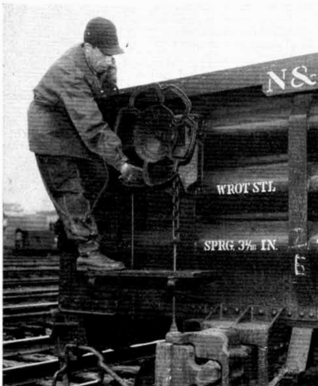
The proper way to set a power brake is being demonstrated by A. L. Mele, yard conductor. The idea is to brace your feet properly, hold the ladder rung firmly with your left hand and pull with your right hand.
