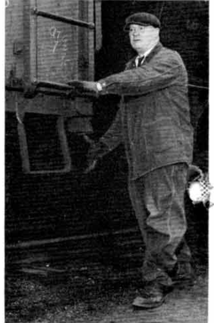
How to cut cars is demonstrated by W. F. Joyce, yard conductor. Face direction in which train is going and run alertly along the ground. Do not cut while riding adjacent car.
