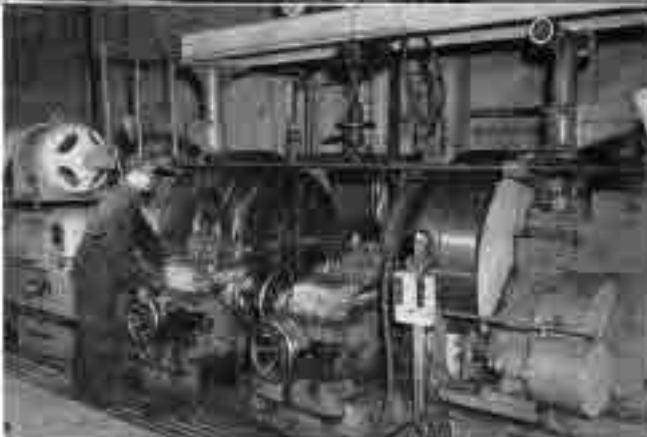
On a wheel lathe, Fred Schwab, machinist, turns car wheels. Although it is large, the lathe is very accurate
