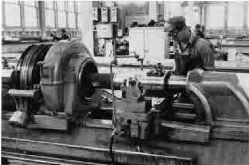
Carman Rich turning the axles on a lathe to fit new wheels. This is exacting work
