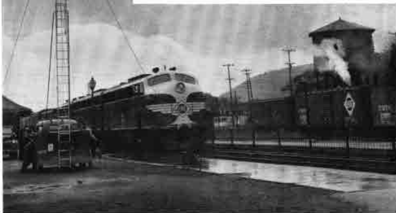
The temporary antenna is completely erected in 12 to 15 minutes ready for reception from any radio equipped train operating within the territory. Train 7 is shown here passing the test unit at Olean, N. Y.
