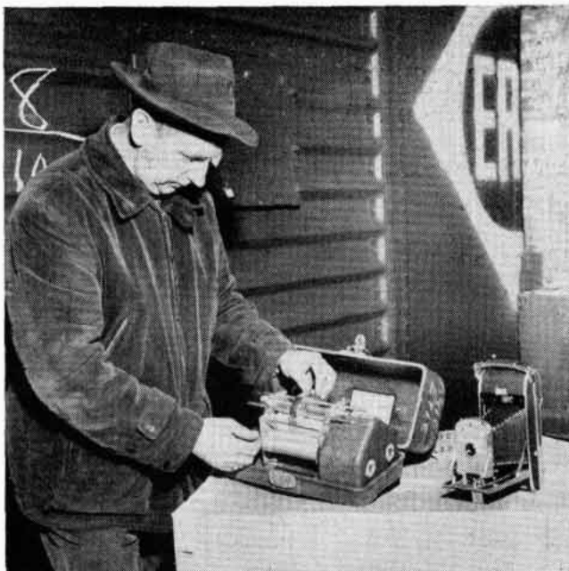
foreman at Cleveland's Scranton Rd. freight house, prepares to use an impact recorder and camera. The recorder is used to check speeds at which cars are switched, and the camera is used for permanent records of damage to freight and as example of what not to do with freight.
