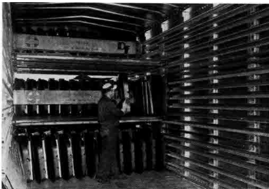
THESE AUTOMOBILE DOORS will have a safe and secure ride, without any dunnage, over the Erie when this car is completely filled. This is a DF car.
