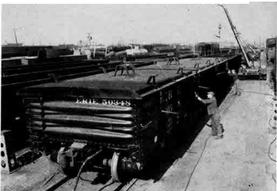
THIS FLAT-ROOF STEEL COIL CAR is the latest model for shipping coiled strip and sheet.
