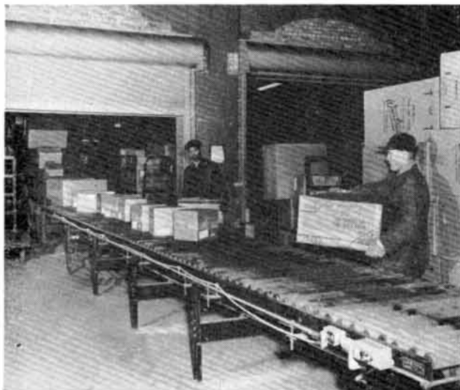
Trucks with packages destined for second floor sorting are unhooked from tow-veyor and placed on conveyor "feed" on first floor. The packages then rise to the second floor on the incline.
