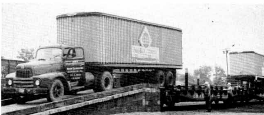
At Hammond, Ind., a truck tractor backs a trailer up the ramp and onto one of Erie's modified flatcars, showing how the trailers are loaded on the cars.
