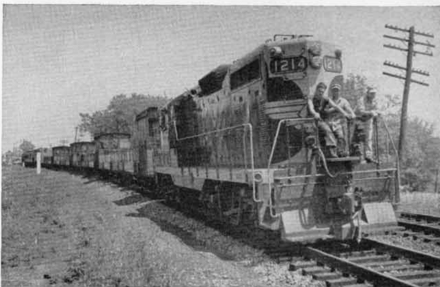
The rail grinding train slowly moves along smoothing our main line rails between Leavittsburg and Akron, Ohio, on the Kent Division.
