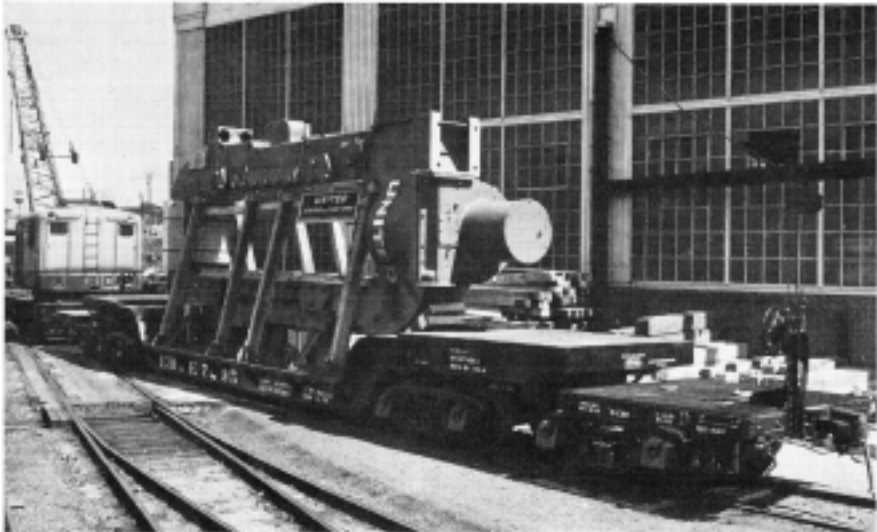
FIRST LOAD FOR THE ERIE'S new ZOO-ton depressed center flat car was this mill housing destined for Japan. Shown outside the United Engineering & Foundry Co.'s Youngstown plant, car and load weigh over a half-million pounds.
