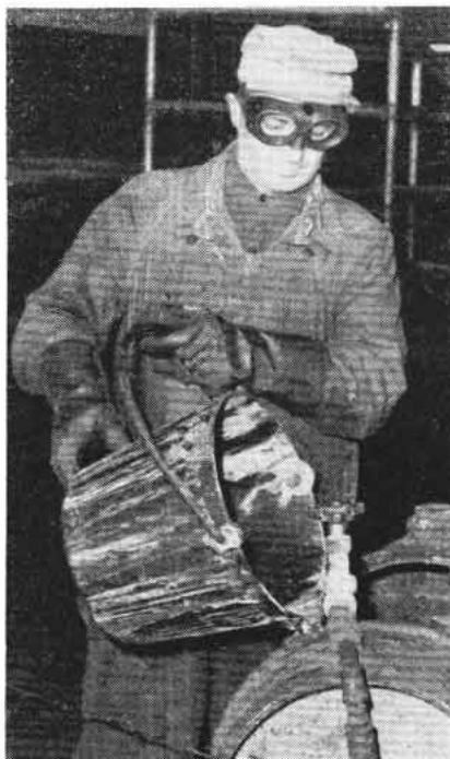
Above, William Bacon wears a dust hood for eye and throat protection. He is cleaning electrical equipment with a corncob blasting hose. Fresh air is pumped into the hood.
