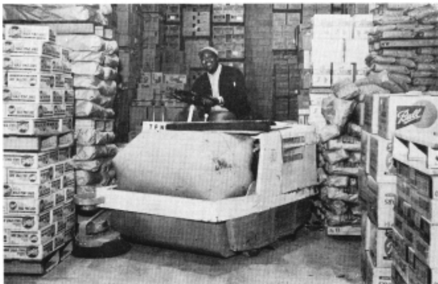
EVEN THE SWEEPING IS FULLY MECHANIZED' and the vacuum cleaner pilot sits down and rides at his work.
