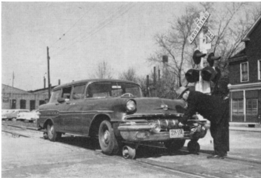
ALONG THE DIVISION THE SUPERINTENDENT'S rail car is known as the Green Hornet. It can be converted from highway vehicle to rail inspection car or back again in less than a minute. Here Harry R. Buchert, operator, sets it on the track.
