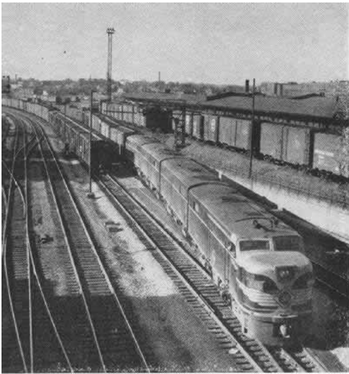
Leaving the longest part of the train on the main track, the engine of Train No. 100, "The Flying Saucer," backs the piggyback cars it pulled to Akron past the freight station toward the piggyback tracks.
