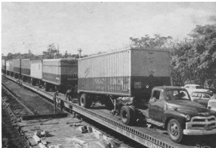
The second phase of the new piggyback operation at Akron is shown here as the trailers from Chicago are hauled off the cars by truck tractor.
