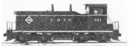
CLASS MARKS ON THIS switcher show that it was built by Electro-Motive Division of General Motors Corp. for yard service.
