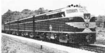
BUILT BY ALCO , this freight locomotive is an FA-15.
