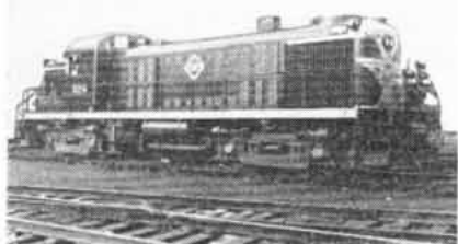
MPSA-16's LIKE THIS may pull commuters, shift freight in a yard, or take out passenger or freight trains along the road. They have steam generators for supplying heat to passenger cars.
