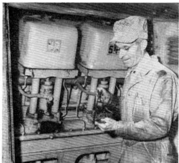
The crankcase oil in one of the diesel switchers was being checked by R. F. Gareri, machinist.
