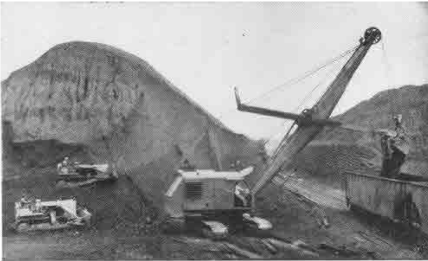
Shown at work here is the new shovel which loads cars with ore at our North Randall, Ohio, ore storage dock. The shovel replaces the ore handling bridge which was blown down during a severe wind storm. The bull-dozer shovels the ore to the shovel which picks it up and dumps it in the cars.
