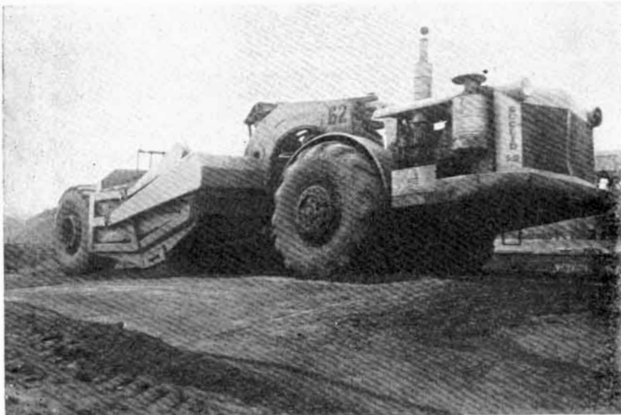
AS THE SCRAPER PASSES over the storage pile it releases its ore from underneath.
