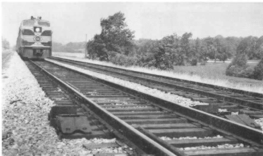
TRAIN NO. 74 approaches the detector's viewing units, which are protected by heavy pieces of timber bolted to the ties.
