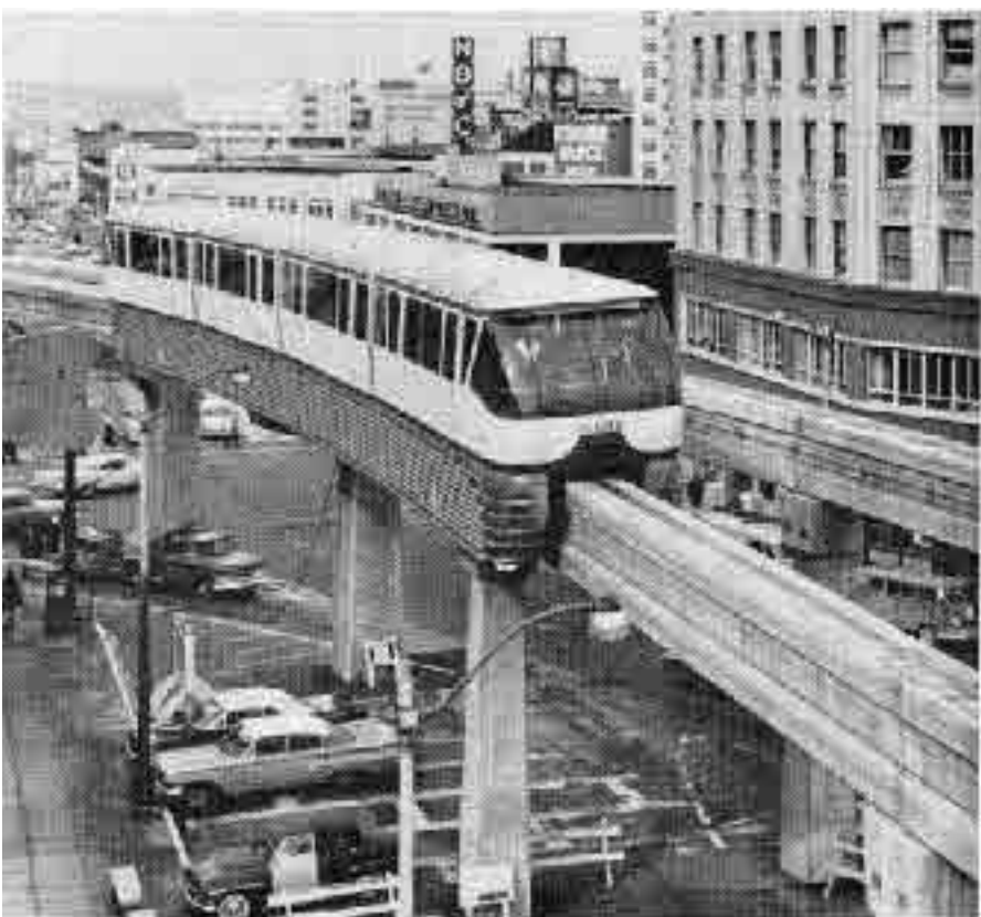
Here's the first train in service 21 feet above Seattle's streets. By the time you read this, second unit will have been tested and put into service. Train of 4 cars carries 450 passengers each trip.
