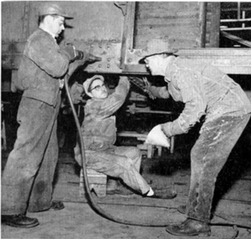
DOOR POSTS ARE REINFORCED. Here Daniel Rinaldi, carman, handles the riveting gun while Arthur A. Catalano, helper, bucks the rivet. Julius Nagy, carman, holds the rivet catcher.
