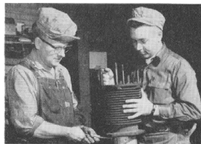
WILLIAM ROSS (L), machinist, and WILLIAM MILLER, machinist apprentice, both of Marion diesel shop, are dismantling freight engine air compressor.
