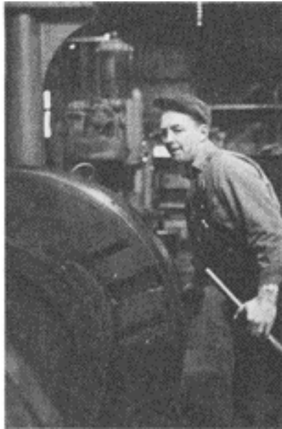
CHARLES CRANDALL, machinist, Hornell diesel shop, is placing a set of wheels in the giant lathe to reshape the tread and flange contours.
