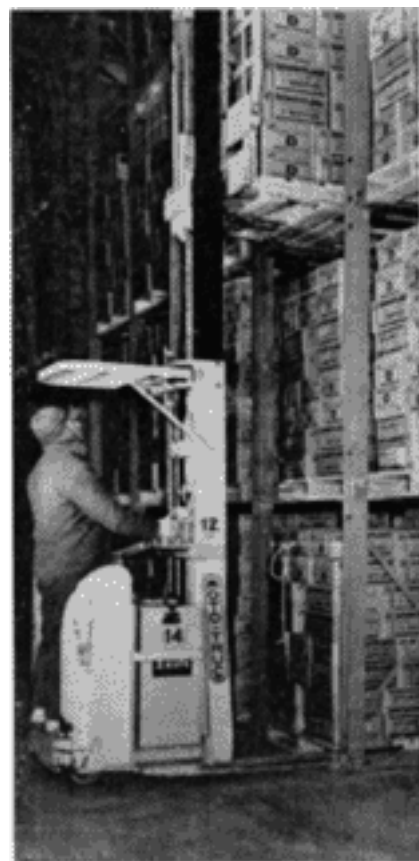
GIANT DEEP FREEZE requires high-stacking fork truck to reach 22-foot storage level.
