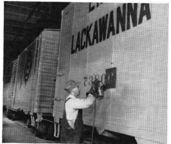
10 At last! George Palmer presses the trigger on his spray gun, and long, sweeping strokes transform one more completed boxcar into a gleaming, gray addition to our fleet. Add the distinctive maroon herald and car markings, and the men at Meadville have made another car ready for the road.
