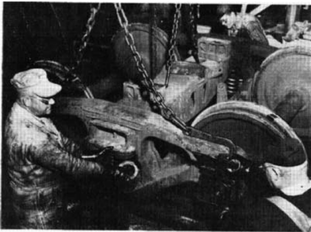
7 Off-line, in the truck shop, while work progresses on car body exteriors and interiors, men are busy rebuilding trucks. These men are installing new springs designed for heavier car loading. Left foreground is P. W. Waid and right is E. N. Macdonald. On other side of truck is R. W. McCracken, Jr.
