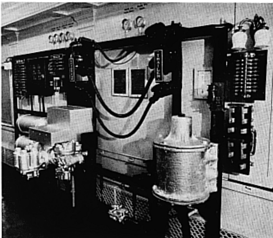
This is the multiple-unit brake and electrical equipment installed in the car, including controller jumpers for both motor car and trailers.
