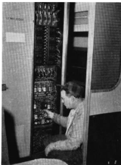
Heart of the air-conditioning equipment is this double-bulb mercury thermostat. Below Pat Cervino adjusts outside selector relay on panel inside car.
