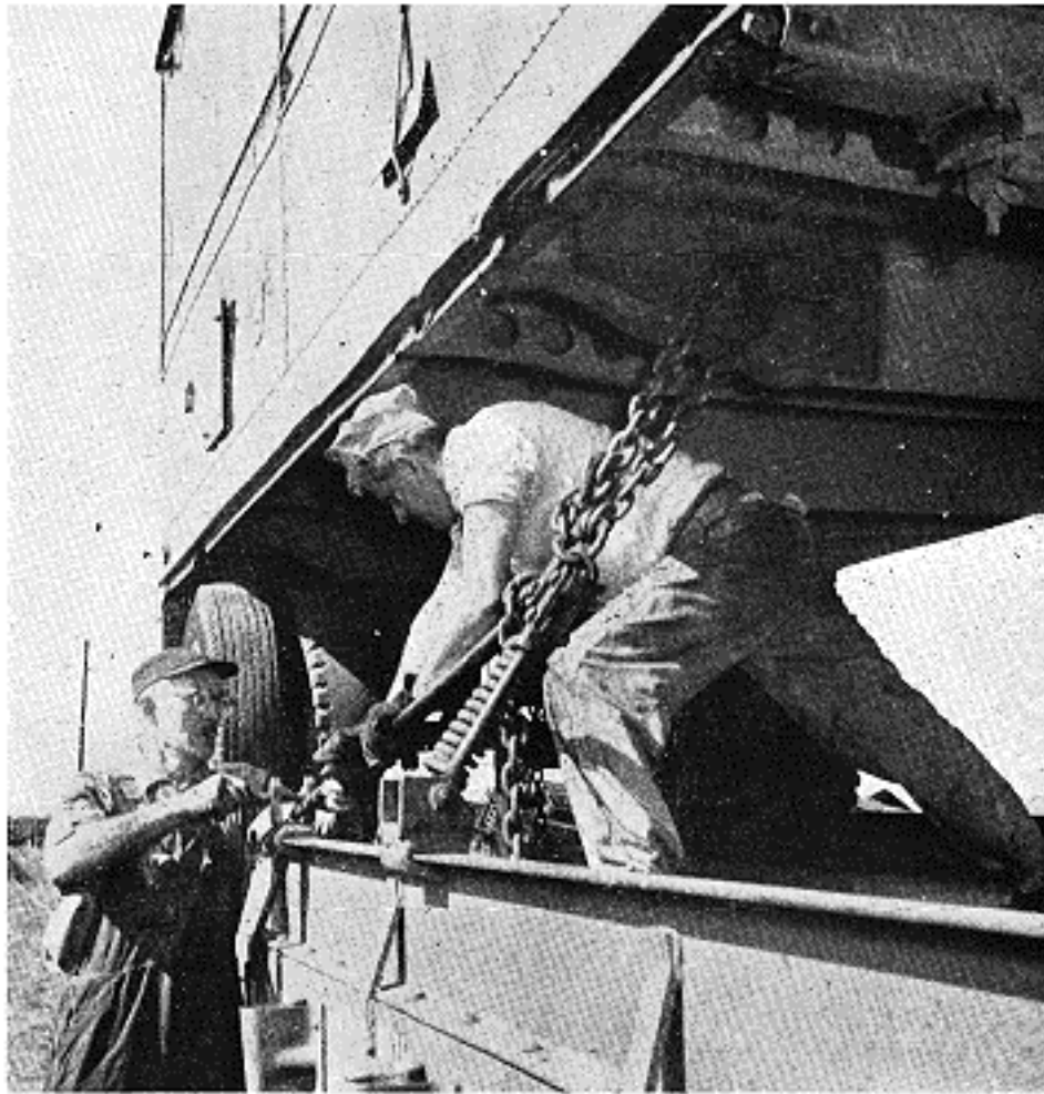
Joseph H. Gaff, leading car inspector at Secaucus, N. J., and John D. Marinzulich tie down side hangers on "Piggy-Back" trailer mounted on flat car.
