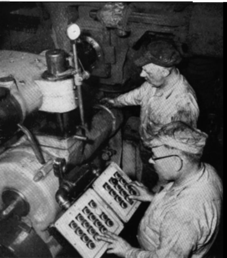
Machinist Helper Wilfred Bartlett and Machinist R. C. Snelson, Jr., set up wheel truing machine preparatory to cutting wheel on "300" series car.
