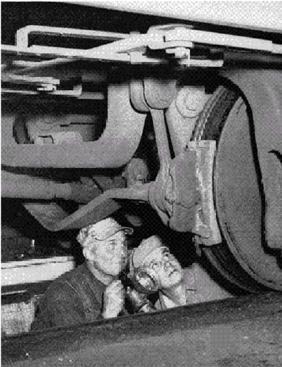
Richard Schultz (left) and William Miles, car repairers, check brake rigging on "300" series car as part of Progressive Maintenance Program.
