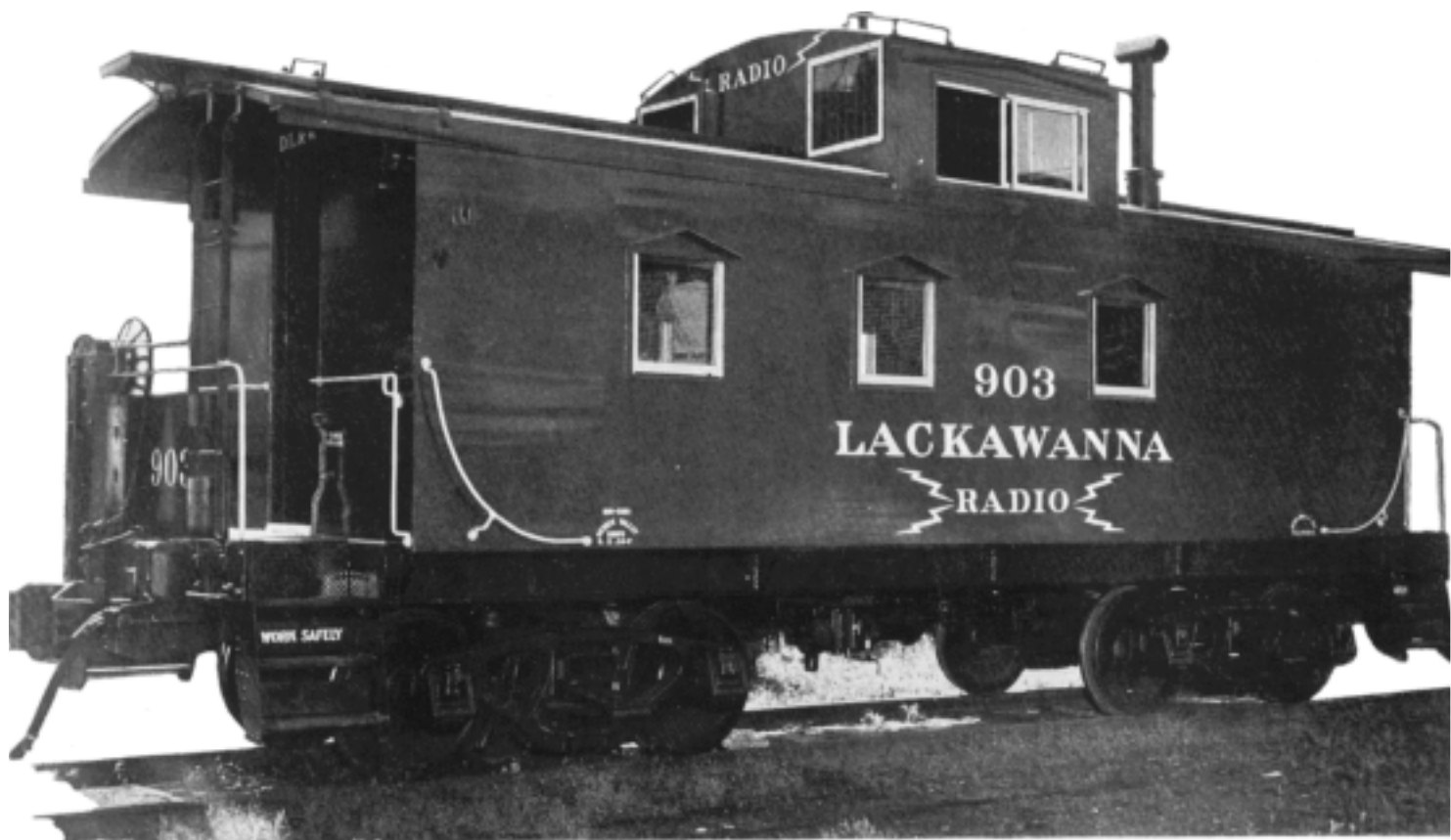
Caboose No. 903 was electric-lighted and radio-equipped.
