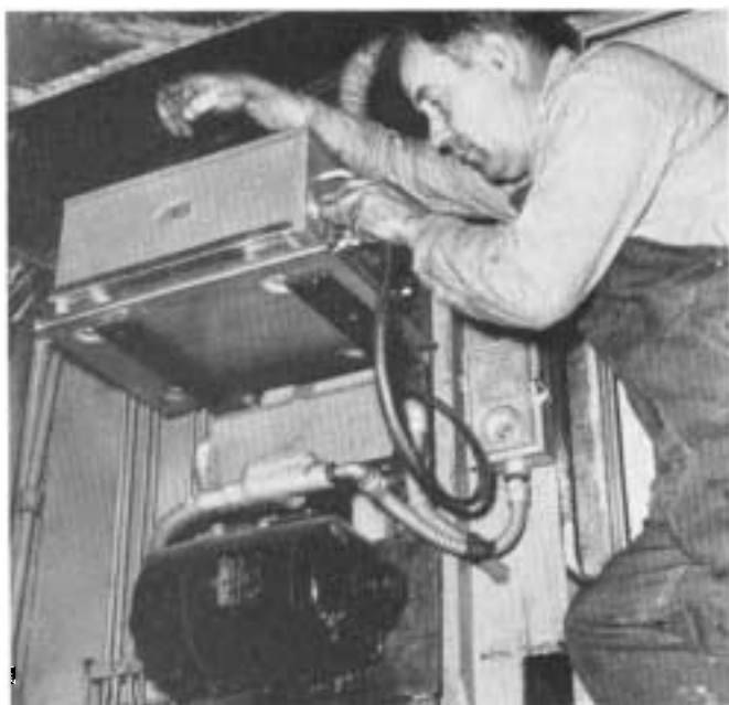
This is the radio installation in Lackawanna diesel locomotives. Stanley Samoles, electrician at Scranton, plugs in the cable to cab.
