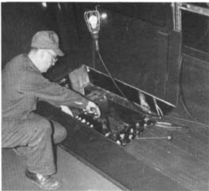
Power for radio in caboose comes from generator-alternator, being installed here by William Hogan, leadman electrician at Keyser Valley.
