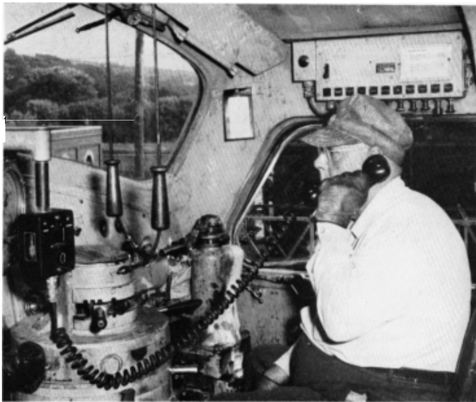
Engineer L. W. Pritchard, of Buffalo division, uses the radio installed in cab of his locomotive pulling BH-4.
